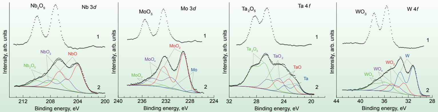
1 — surfaces of virgin higher oxides; 2 — surfaces of higher oxides after  $\text{Ar}^+$  ion bombardment ( $E = 3 \text{ keV}$ ;  $D \approx 3 \times 10^{17} \text{ cm}^{-2}$ )
