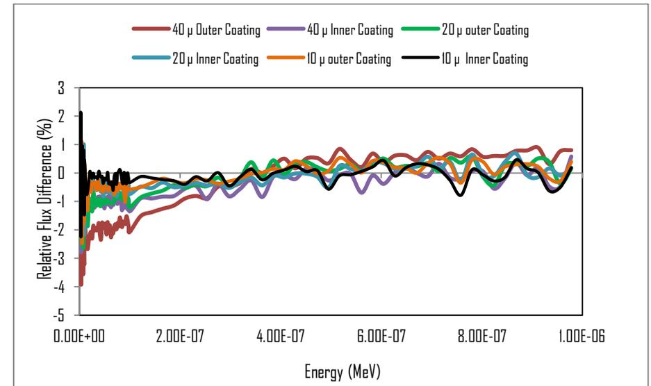
Neutron Flux for inner-side coating and its comparison with external coatings flux changes
