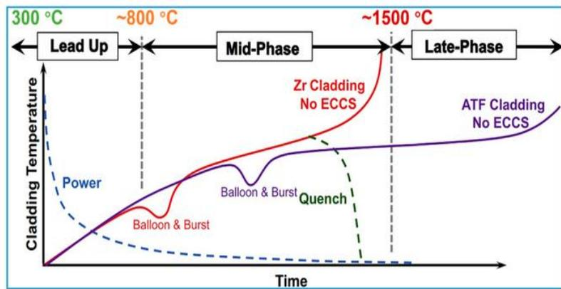
Potential delaying effect of accident-tolerant fuel (ATF) cladding [1]
