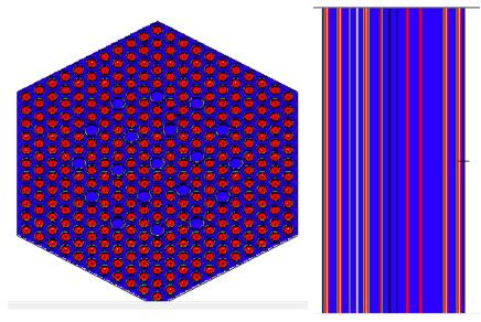
2D Reference VVER-1200 Fuel Assembly as generated by MCNPX
